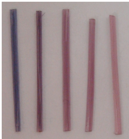
FIGURE 3. Photographs of alginate bundles (1 in. long) with embedded PCDA liposome dried after \text{CaCl}_2 baths. From left: 0%, 1%, 3%, 5%, and 10%.
